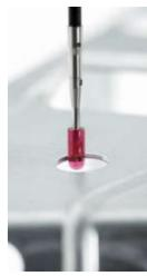
Cylinder styli e.g. for measurement of metal sheets
