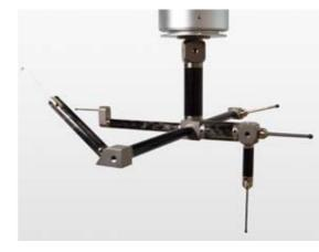
A complex stylus configuration with multiple components
