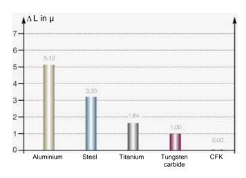
Thermal length increase in  $\mu$  with a 200 mm probe extension and a temperature difference of 1K
