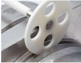
Disc stylus for measuring edges or undercuts
