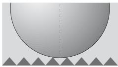
Probing with such a large diameter ball can average out the effects of very rough surfaces
