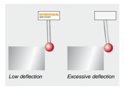
Deflection has a direct impact on the accuracy of measurement
