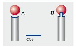
A: Cap connection, less gluing area
