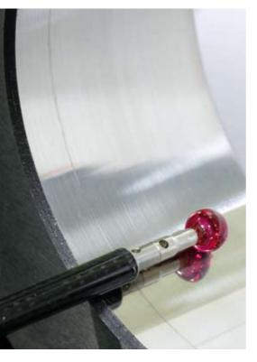
To stay competitive, manufacturers have been continually upgrading their co-ordinate measuring machines. CMMs are now being integrated directly into manufacturing as part of production processes and swift, high-performance scanning systems guarantee extremely precise measurements within the tightest timeframes.
