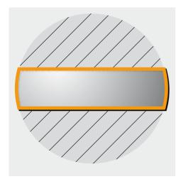
The edges of all discs are curved, as though a section had been cut out of a sphere at its equator.
