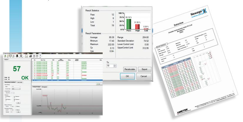
DataView® software is an easyto-use data acquisition utility that is compatible with all Newage or competitive hardness testers having an RS232 serial data output and capable of ASCII transmission. DataView® is designed to enhance the capabilities of hardness testers by allowing you to transfer test results directly to a PC for real time, on-screen data management.
