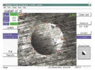
impression roundness and overall surface finish. The powerful PC based B.O.S.S.® features Windows-based software, integral statistical functions, data storage and transfer, several different report styles and advanced options. These include real time advanced SPC; the ability to save the viewed image; and a manual measurement function that allow the B.O.S.S.® to be used to measure other visually discernable aspects such as etched case depth layers.
