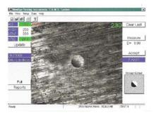
anomalies as impression roundness and overall surface finish. The powerful PC based B.O.S.S.® features Windows-based software, statistical functions, data storage and transfer, reporting function and an assortment of advanced options. These include real time advanced SPC; the ability to save the viewed image; and a manual measurement function that allow the B.O.S.S. to be used to measure other visually discernable aspects such as etched case depth layers.
