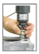
With the B.O.S.S.® Brinell impressions are measured in a matter of seconds and yield a measurement resolution of 0.01mm. The B.O.S.S.® even takes into account such
