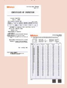
A Certificate of Accuracy, traceable to the NIST, is furnished with each MITUTOYO gage block set and individual block
